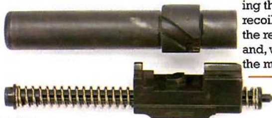
The Cougar 8000 uses a rotary barrel locking mechanism. The central block's "tooth" travels in a cam track in the barrel's bottom lug.
